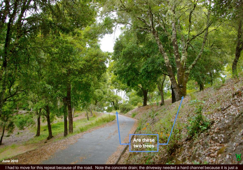
I had to move for this repeat because of the road. Note the concrete drain; the driveway needed a hard channel because it is just a skin of extra fine chips on base-rock sealed with oil (oil works well here on a hard base, if one maintains it). The County road, although of poor original construction, has been there for 150 years, paved for the last 40 with but 3/4" of oil and screens on bare dirt.
